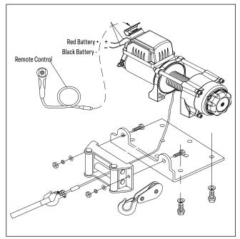
1. Your winch is designed with a bolt pattern that is standard in this class of winch. Many winch mounting kits are available that
