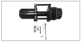
1. Prepare the suitable fittings: 5MM Internal Hex wrench, 10MM Open End wrench, as shown in photo.
