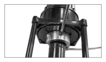
7. Use wrench to screw in M8 X 15bolt from the top hole.
