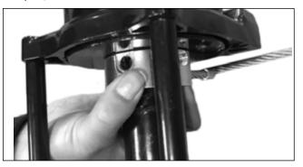
3. Press the clamp to the drum and make sure the rope is in the groove of clam. Adjust to the same position of holes in clamp and drum.
