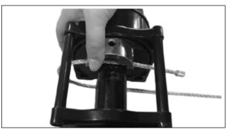
2. Adjust the drum to make the screw hole on the top, put the rope on the drum and put the clamp on the rope (the hole close to casting plate)
