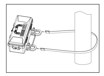
Utility winch can be used in a portable fashion by using the supplied straps and shackles.
