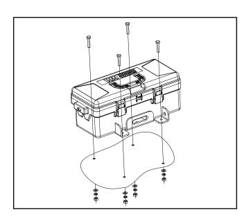
Using M10 mounting bolts, washers, and nuts, tighten the mounting hardware.
