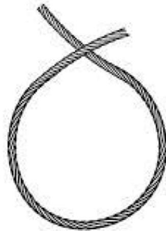
Fig. B This wire rope is kinked. It is too late to reverse the damage at this point, the wire rope must be discarded. It is permanently damaged and must not be used.
