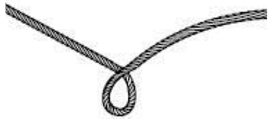
Fig. C This is a kinked wire rope that has been straightened out. Even though it has been pulled straight, some wires in the wire rope are stretched, and others are severely bent, if not broken. The unstretched wires will take more load and can fail suddenly before the rope reaches its capacity. This wire rope must be discarded and not be used.
