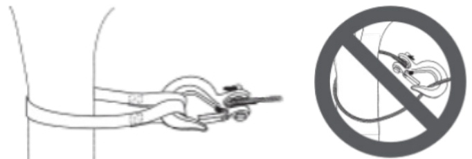
Figure E - Using a strap anchor point
