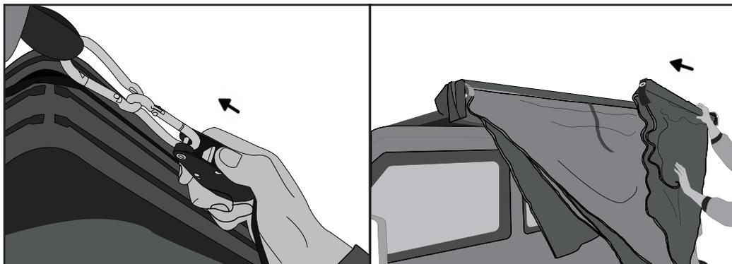
Use the quick release ratchet ratchets to release the front and rear tension ropes, then swing the arms back into the closed position. The canvas should form a triangular shape. |
