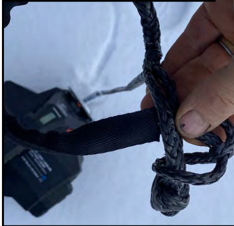
Figure 22b –Next loop the choking end back over the choking knot
