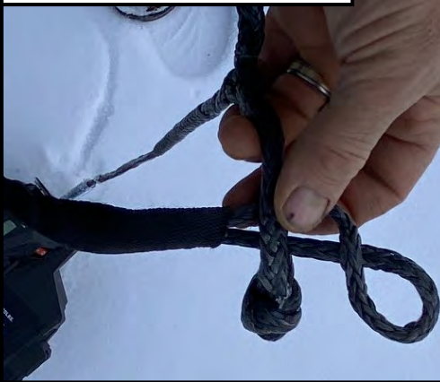
Figure 22a –First thread the choking end through the loop beneath the choking knot
