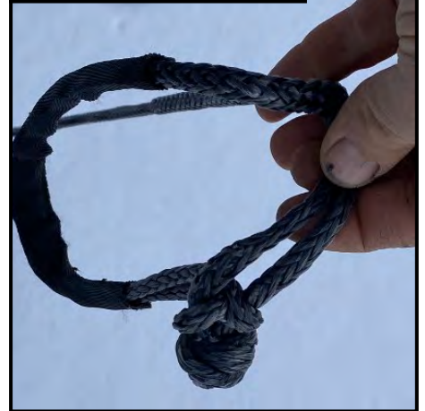
Figure 22c –Pull the soft shackle tight to secure
